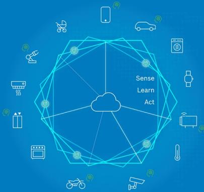
An edge computing solution typically sits between the IoT devices, the gateways to connect the devices, and the IoT cloud platform. The basic features of an edge solution focus on connecting the devices, processing and managing the data locally, and moving data to the cloud platform for further data analytics and integration with back end services.
