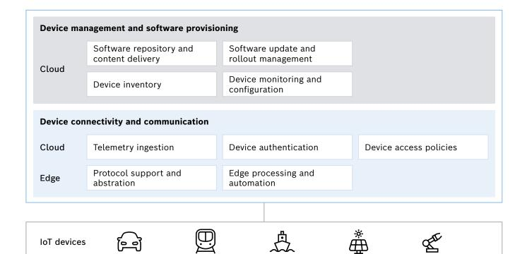
From edge to cloud: principal building blocks for device connectivity in the IoT
